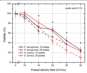
**Fig. 3** The inactivation of bacteria using pulsed electric field treatment combined with acetic acid (0.1%). The treatment was efficient for both bacteria, which was unachievable during separate exposures. The asterisk (\*) represents statistically significant difference (P < 0.05) versus control (chemical treatment only)
