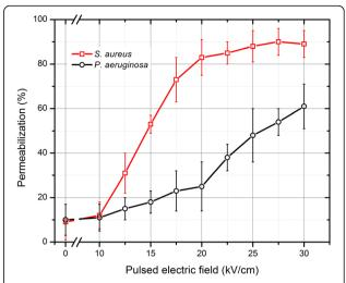
**Fig. 1** The permeabilization of *S. aureus* and *P. aeruginosa* during pulsed electric field treatment. The *S. aureus* was more susceptible and the  $20 \text{ kVcm}^{-1} \times 100 \text{ µs}$  protocol induced a saturated (> 85%) effect
