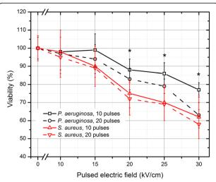
**Fig. 2** The dependence of *S. aureus* and *P. aeruginosa* viability on the applied pulsed electric field parameters. Higher number of pulses resulted in higher loss of viability for both bacteria, however the effect was more profound (P < 0.05) in the *P. aeruginosa* case. The asterisk (\*) represents statistically significant difference (P < 0.05) versus control (non-treated samples) for both bacteria
