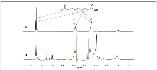
Fig. 2 <sup>1</sup>H-NMR studies of Azelaic acid. Spectra of a solution of standard azelaic acid (a) and of the azelaic acid extracted and purified from PSA (b) recorded at 25 °C in CD<sub>3</sub>Cl
