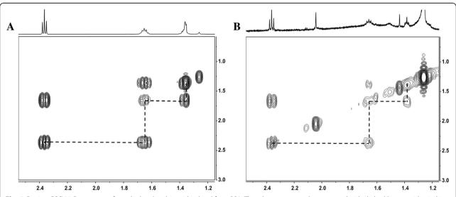
Fig. 3 Depicts COSY 2-D spectrum of standard and azelaic acid isolated from PSA. The relevant cross-peaks, connected with dashed lines, are identical in the standard sample and in the extracted sample (a and b)
