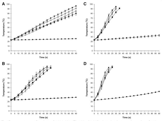
**Fig. 2** Temperature-time curves for apple juice of 18 (**■**), 24 (△), 36 (**▼**), 48 (o), and 72 (•) °Brix during ohmic heating at voltage gradients of 30 V/cm (**a**), 40 V/cm (**b**), 50 V/cm (**c**), and 60 V/cm (**d**). Error bars indicate standard deviations calculated from triplicates
