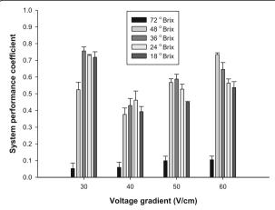
**Fig. 3** System performance coefficient levels for 18, 24, 36, 48, and 72 °Brix apple juice during ohmic heating at voltage gradients of 30, 40, 50, and 60 V/cm. Error bars indicate standard deviations calculated from triplicates
