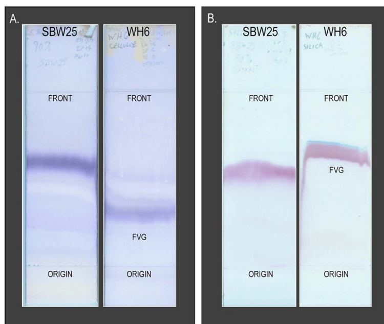
Figure 1 Thin-layer chromatograms of 90% ethanol extracts of dried culture filtrates from P. fluorescens SBW25 and WH6.
