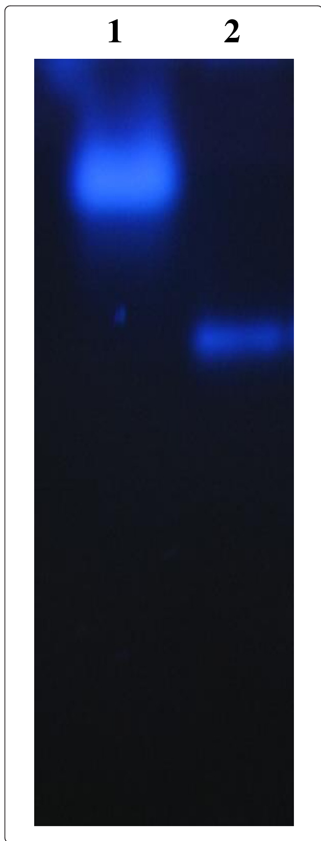
Figure 1 Zymographic analysis of B. pseudomallei leucine aminopeptidase [12]. (8% polyacrylamide gel, 8 V/cm, 120 min.). Lane 1- commercial aminopeptidase I of Streptomyces griseus . Lane 2- concentrated crude extract of B. pseudomallei NCTC 13178; *figure prints in black and white.
