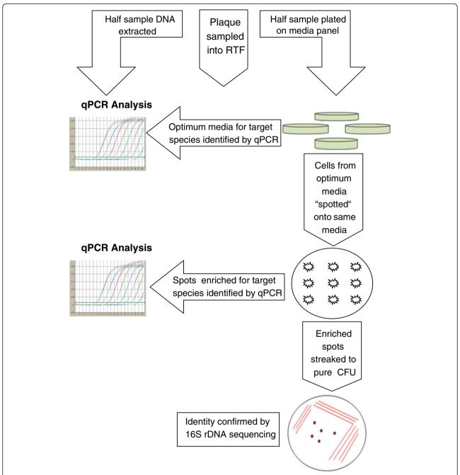
Figure 1 An overview of the screening and isolation process used to isolate target bacterial species. RTF denotes reduced transport fluid and gPCR describes quantitative PCR.
