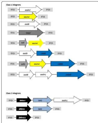
**Fig. 2** Schematic representation of the various cassette arrays found in class 1 and class 2 integrons. The arrows display the open reading frames of the different genes. All *aadA* and *aadB* genes are presented as white arrows, *dhfrA*, *aacA4*, *orfD*, *oxa2*, *catB*, *cmlA6*, *sat2* genes are presented as black, yellow, light grey, grey, blue and light blue arrows respectively. The grey light boxes indicate the 3' and 5' CSs of class1 or class 2 integrons
