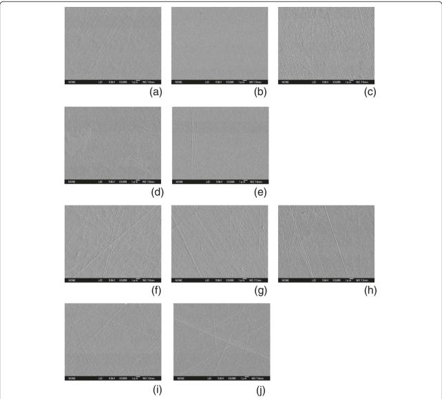
Figure 1 SEM micrographs. The fine group specimens had a relatively featureless surface compared to the coarse group specimens. Fine group: Oxinium (a), Co-Cr-Mo (b), Ti-6Al-4 V (c), Cp-Ti (d), SUS316L (e). Coarse group: Oxinium (f), Co-Cr-Mo (g), Ti-6Al-4 V (h), Cp-Ti (i), SUS316L (j). Original magnification × 5000 (Scale bar = 1 µm).
