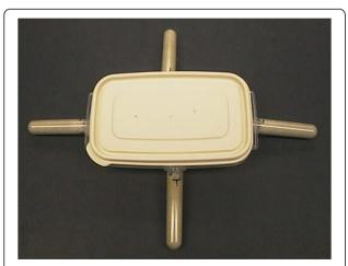
**Figure 4** Bioassay unit composed of a plastic container (14.5 × 8.5 × 4 cm) filled with 100 g of moistened sand, connected to four 14 ml polystyrene round bottom test tubes (17 × 100 mm) containing either treated (two tubes) or control (two tubes) substrate.
